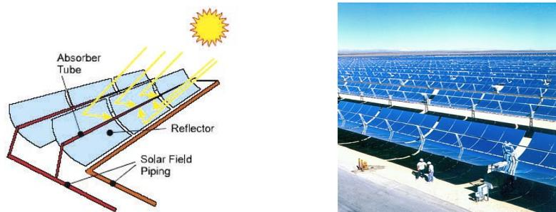
Figure 2. Parabolic Trough CSP System and Parabolic Trough System at Arizona
